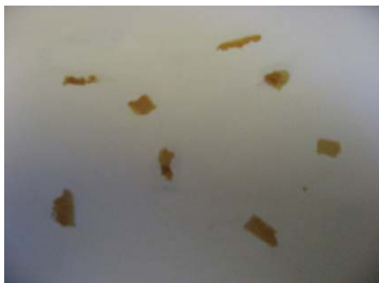
Biofilm release by using TwinOxide®
