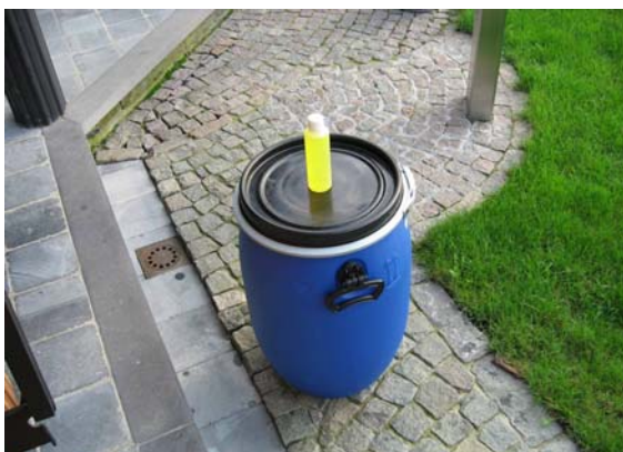
Vessel with cover for stand disinfection of small filters
