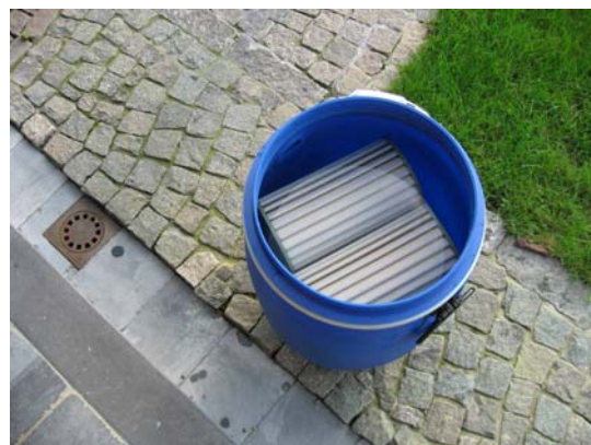
Vessel with cover for stand disinfection of small filters
